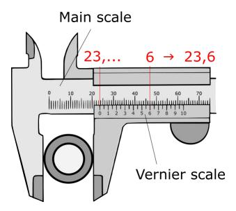
The decimal place is now determined on the vernier scale. The numerical value on the vernier scale is searched for whose scale line lies exactly on the same line as one off the scale lines on the main scale. In the example, this is the value 6 on the vernier scale. This results in a measured value of 23.6.
